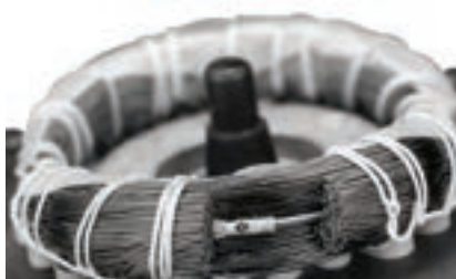
PTC sensor incorporated in windings
