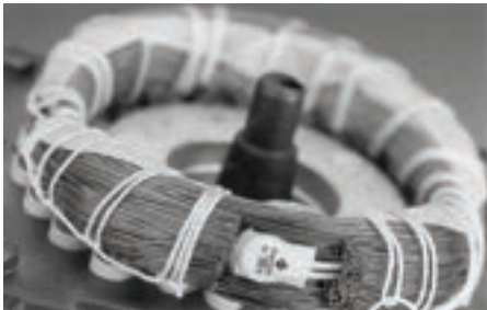
Thermal switch incorporated in windings
